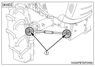
(1) Grease fitting (Tie-rod ends)
