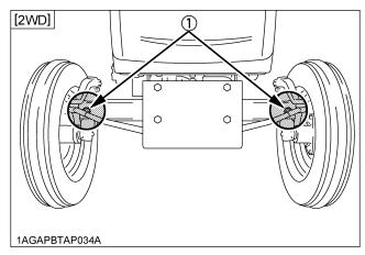
(1) Grease fitting (Knuckle shaft)[RH, LH]
