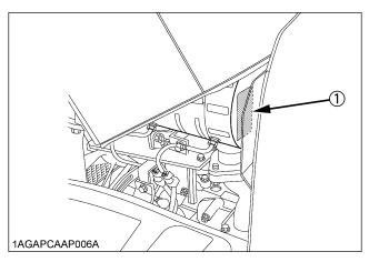
(1) Diesel particulate Filter (DPF) serial number
