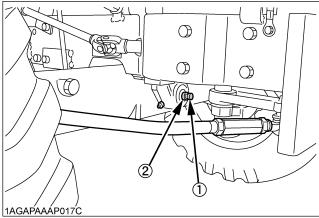
(1) Adjusting screw (2) Lock nut
