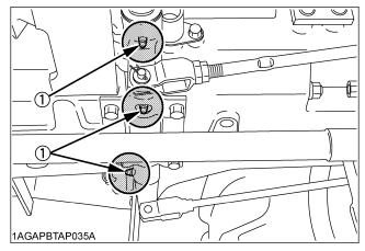
(1) Grease fitting (Pedal shaft)
