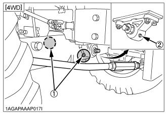
(1) Grease fitting (Front axle support)
